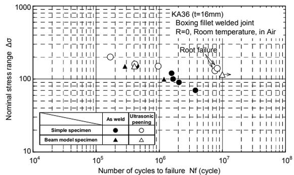
Fig.9 Fatigue test results for boxing weld joints
