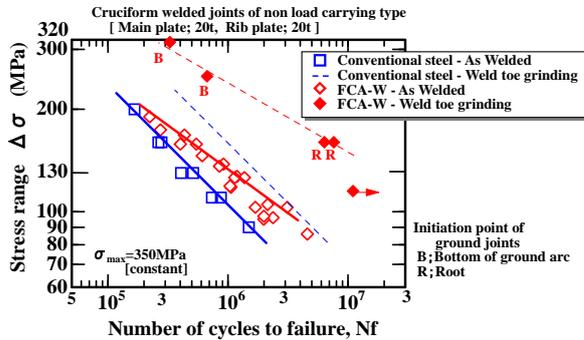
Fig. 4 Results of fatigue test of FCA-W steel with weld toe grinding
