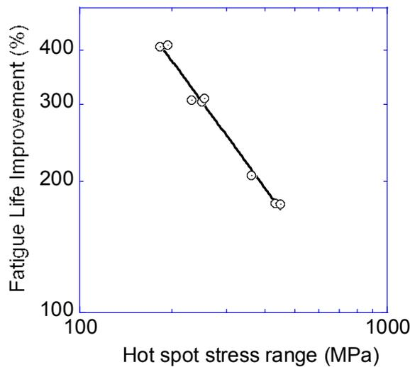
Fig.2 Relations between stress ranges and fatigue life improvement by FCA-W steel application
