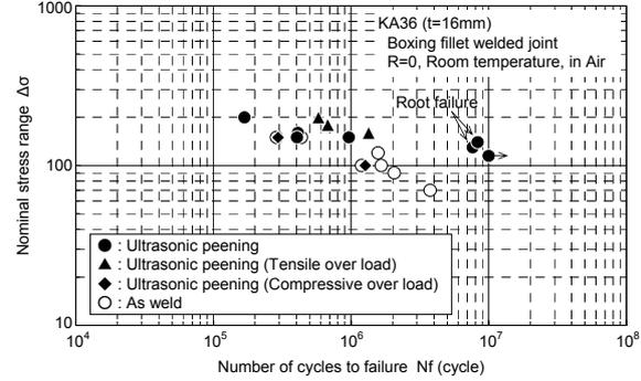
Fig. 11 Effects on over load on fatigue strength
