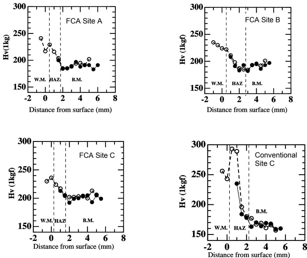
Fig.1 Hardness distribution of welded joints
