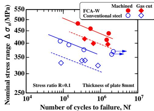
Fig. 5 Results of fatigue test of FCA-W steel for base metals
