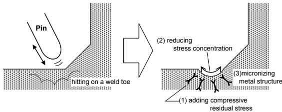
Fig.6 Schematic views of effects by UP-method
