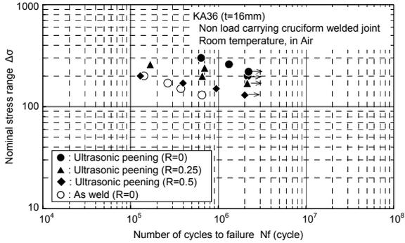
Fig.10 Effects of stress ratio on fatigue strength
