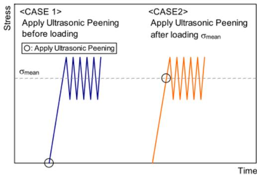
Fig.12 Loading cases for fatigue tests
