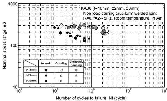
Fig.8 Fatigue test results for fillet weld joints
