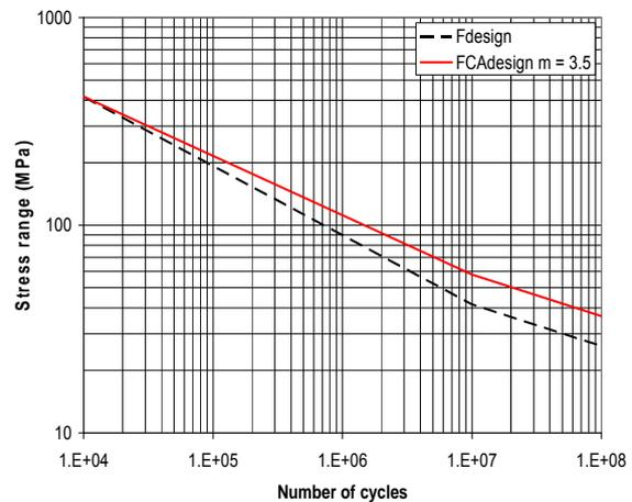
Fig.3 Design S-N curves of conventional and FCA-W steels
